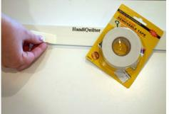
Double sided tape is provided to secure the track to your table. Only one track needs to attach to the table. Cut tape into small sections and adhere to the center of the track. Note: If the HQ II is not being set up to the full length, tape may not be needed as the "L" bracket secures the track at shorter lengths.
