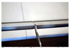
Once the Velcro® has been applied to the tubes, it can be clipped where the poles meet for easy separation when the frame is taken down.
