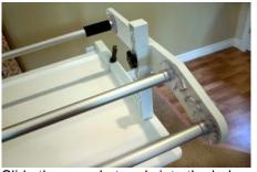
Slide the sprocket ends into the holes on the printed side arm with Y latches. Hold the Y latches up as you push the tubes in so they don't get caught behind the sprocket. The latches and sprockets work together to hold tension on the quilt top and back.
