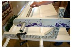
Insert the end of the tubes into the printed side arm that does not have the Y latches. The tube with the foam grip is the single take-up roller.
