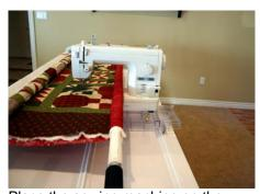
Place the sewing machine on the carriage. Reattach the roller to the sidearm. Evenly roll the take up roller until the quilt top and back are taut. The latches and sprockets will hold the tension.
