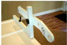
Push the threaded bolt into the vertical guide of the "L" bracket.
