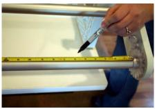
Next, prepare to attach the Velcro® to the tubes. Measure in 6" from each end of the frame and mark if desired.
