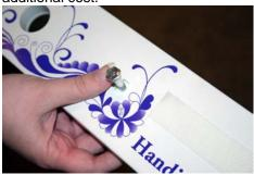
Find the small hole on each of the printed side arms. Thread the bolt through the hole. The bolt head goes against the *flat side* of the arm without the groove.
