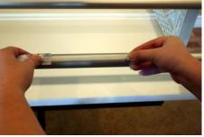
Peel the backing off the Velcro® and apply to all three tubes starting at the 6" mark and ending at the opposite 6" mark. Note: Make sure the Velcro® is straight so the leaders attach correctly.
