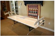
The HQ II should now be set up as shown. The printed side arms should "waterfall" down at the ends. If the side arms are curving up, they're upside down.
