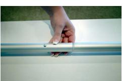
The tubes (take-up rollers) can be connected in combinations of roughly 6, 8 or 10 1/2 foot lengths. Select your preferred length and couple the tubes together by pressing the snap button and pushing the tube inside the adjoining tube until the pin pops out.
