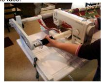
Remove the single take—up roller and slide it under the neck of your sewing machine.
