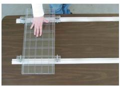
Place the bottom carriage (without handles) on the first track. Set the second track down under the wheels for placement. Once the tracks are aligned, the "L" brackets can be clamped into place.
