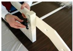
Push the threaded bolt into the vertical guide of the "L" bracket. Thread the black knob on the bolt and tighten. You will adjust the arm up or down with the knob once you get the guilt loaded.
