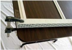
Place the "L" brackets on the tracks at each end of the table. (Shown above.) If tracks are longer than the table, it will not damage them to let them hang over the edge.
