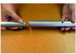
The tubes (take-up rollers) can be connected in combinations of 6, 8 or 10 foot lengths. Select your preferred length and couple the tubes together by pressing the snap button and pushing the tube inside the adjoining tube until the pin pops out.
