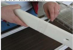
Find the small hole on each of the white side arms. Thread the bolt through the hole. The bolt head goes against the *flat side* of the arm without the groove.
