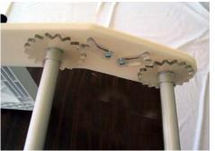
Slide the sprocket ends into the holes on the white side arm with Y latches. Hold the Y latches as you push in the tubes in so they don't get caught behind the sprocket. The latches and sprockets work together to hold tension on the quilt top and back.
