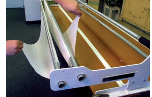
1.17 Matching leader center marks to pole center marks, begin attaching the leaders to the Velcro®, working from the center to each end of the Quilt Top pole and Backing pole so they hang to the center between the poles.
