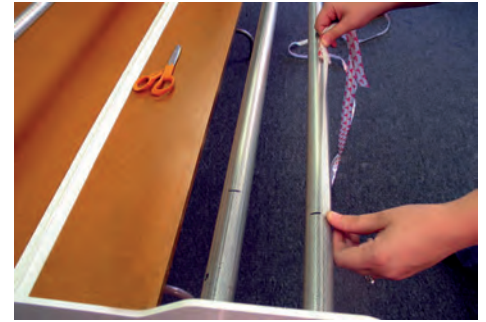
1.14 Peel the backing off the Velcro® and apply to the Take-up pole, starting at the 6" mark and ending at the opposite 6" mark. Use the snap buttons as a guide to keep the Velcro straight. It is recommended that you place the Velcro in a line below the buttons.
