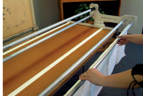
1.16 A set of 9 1/2' marked leaders are provided with this frame. Fold each leader in half lengthwise and mark the center.
