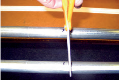
1.15 Once the Velcro® has been applied to a pole, it can be clipped at the couplers to enable disassembly. If you don't intend to change the size of your frame, the Velcro® can be left uncut.
