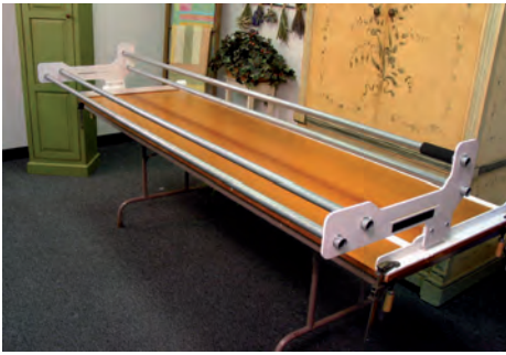
1.12 This photo shows the frame set up at 8'.
