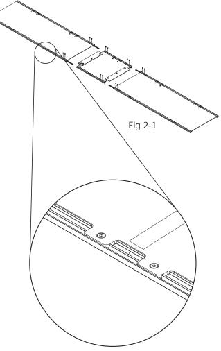
Detail 2-1 - Table shown upside down with nonadjusting track support at front edge of table
