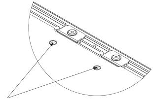
These screws do not turn, they have flats for adjusting bracket – do not turn. Tighten at the acorn nut only.
