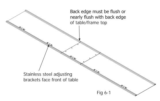
**6-2:** Study where the new black plastic top will be aligned on the frame with it as flush to the back edge as possible, and install the new tape on the perimeter and on all cross members to hold down the new plastic top.
