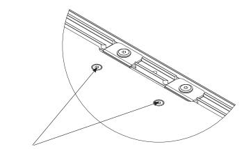
These screws do not turn, they have flats for adjusting bracket – do not turn. Tighten at the acorn nut only.
