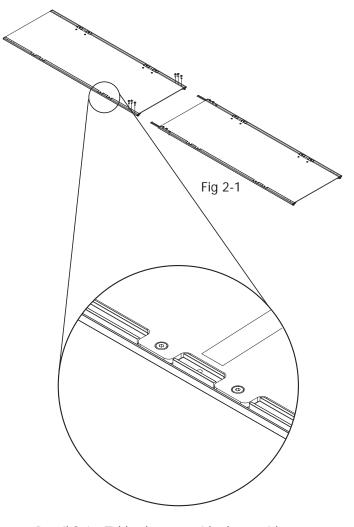
Detail 2-1 - Table shown upside down with nonadjusting track support at front edge of table
