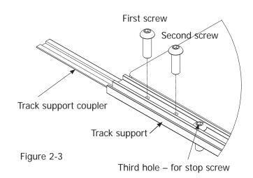
2-4: Insert a coupler into each of the two track supports on the first table top assembly up to the stop screw. Thread an M5x8mm Socketed Button Head Screw into the first and second holes on both track supports on the first table top assembly and lightly tighten. (Fig. 2-4 and Detail 2-4)
