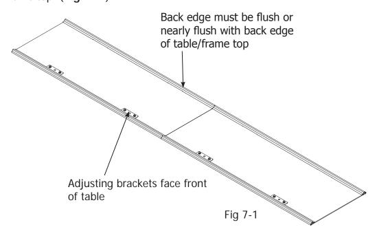
HINT: On the Adjustable Table the aluminum track support should be no more forward than the inside edge of the protective edging on the table top (about 1/8"). On the QuilTable the aluminum track support should be no more forward than the inside radius of the QuilTable Frame (about 1/4"). This is important so the carriage encoder will not interfere with table top assembly and will operate correctly.
