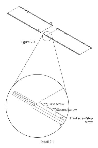
**2-6:** Slide the second table top assembly over to receive the two couplers, align the couplers and slide the two table top assemblies together as close as possible. There should be minimal gap. Hold the two adjoining track support sections tightly together and thread an M5x8mm Socketed Button Head Screw into the first and second hole on the two track supports on the second table top assembly and lightly tighten. (**Fig. 2-5**) You may need to gently rock the track support to seat the coupler.
