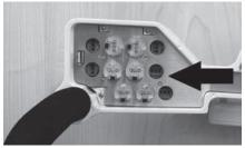
3. Remove any lights that may be in the innermost three slots on both sides of handlebars and place them in empty slots according to your preference
