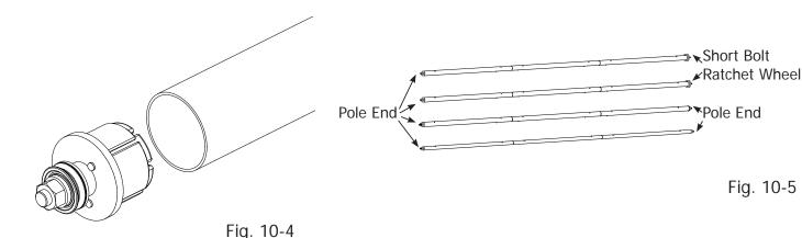
**10-5:** Slide one pole end into the end of one large 12-foot pole assembly, as shown in Fig. 10-4. Check that the pole end is inserted completely into the pole assembly.
