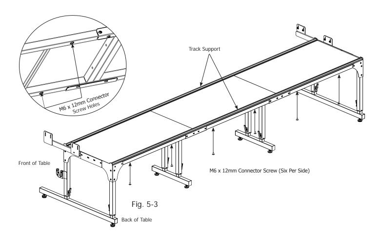
**5-6:** Place the machine onto the carriage and again, roll it the entire length of the frame, working the tracks into the wheels as you go. Lightly tighten the front track support screws as you move down the table. Check the carriage to verify that it rolls smoothly and that both ends of the carriage are engaging the tracks.
