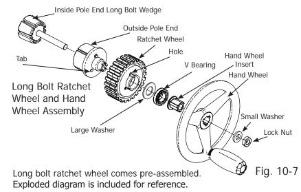
**10-18:** In same manner, slide the long-bolt ratchet wheel and hand wheel assembly into the open end of the remaining pole assembly and tighten the nut, using the 13/17 mm wrench. Check to be sure the hand wheel engages the ratchet wheel assembly and does not spin loosely shown in Fig 10-7. This completes the take-up pole show in Fig. 10-9.
