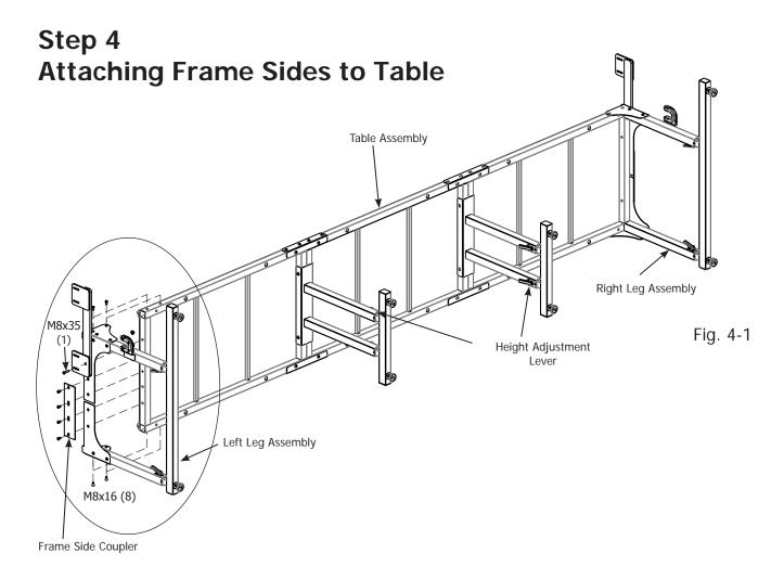
Note: Finger-tighten screws only until all screws are in place. They will be tightened after the table is uprighted once again. See step 4-9.
