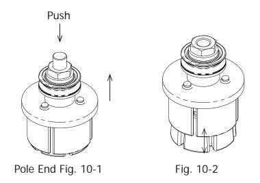
**10-4:** Repeat **steps 10-1** through **10-3** to prepare the 5 large pole ends and the 2 small pole ends for insertion.
