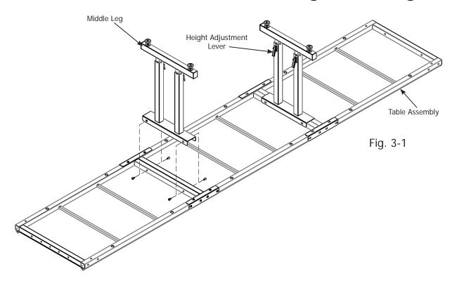
Note: If instructions were carefully followed in Section 2, there should be minimal gap between the table sections where the sections meet. The middle leg/s should slide over the two table section end tubes easily. Check to ensure that all table splice brace screws are tightened before tightening the four middle leg screws.
