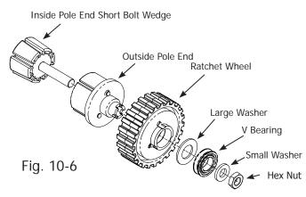
Short-bolt ratchet assembly comes pre-assembled. Exploded diagram is for reference only.
