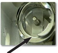
Apply one drop of Lube #6 (Purple), to the raceway of the bobbin case support two to three times per day. This application is based upon sewing for 8 hours of machine time. If the machine is used less, lubricate the hook less frequently. After the lubrication of the hook, it is recommended that one momentarily sew on scrap material before resuming the sewing of the quilt. Failure to do so may result in oil stains on the quilt.
