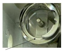
Apply one drop of <u>Lube #6 (Purple)</u>, to the raceway of the bobbin case support two to three times per day. This application is based upon sewing for 8 hours of machine time. If the machine is used less, lubricate the hook less frequently. After the lubrication of the hook, it is recommended that one momentarily sew on scrap material before resuming the sewing of the quilt. Failure to do so may result in oil stains on the quilt piece.
