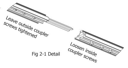
**NOTE:** The exisiting four-foot track supports may have only two coupler screw holes instead of three.
