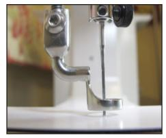
Note that there is too much gap between the bottom of the foot and the needle plate.
