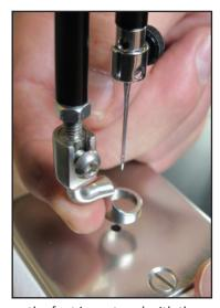
3. Ensure the foot is centered with the needle when the foot is fully tightened with the 2.5mm hex wrench. If it isn't properly centered, loosen the lock nut; center the foot with the needle; hold the foot in position; and firmly tighten the lock nut.
