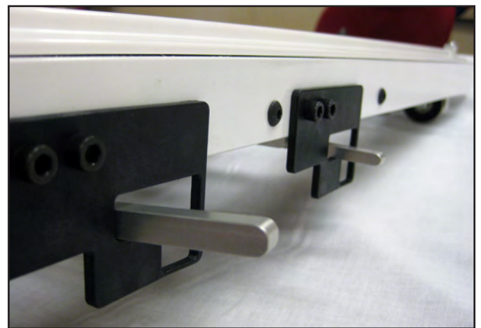
Figure 3.61 Levers Up = Gear Disengaged / Free Motion
