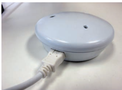
Figure 5. Charging cable installed. Note flat on cable is up.
